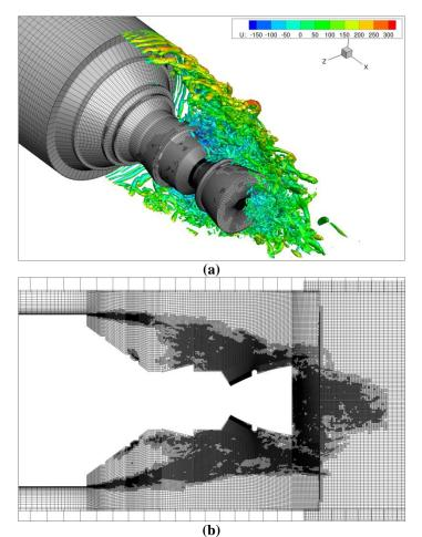
**Fig. 1** Ariane 5 model buffeting using a  $k - \varepsilon$  HRL model and an AMR method. (a): Q criterion colored by axial velocity. (b): slice of the AMR overset meshes in the recirculation area
