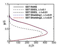
Figure 1: Eddy-viscosity ratio in a flat-plate boundary layer for different grid spacing to boundary-layer height ratios. Comparison of RANS, DDES and new shieldings
