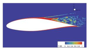
Figure 2: Application of the new shielding function to a stalled airfoil
