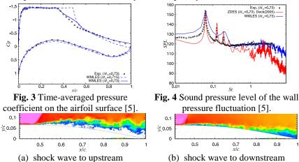
**Fig. 5** Snapshots of instantaneous streamwise velocity distribution  $u/u_{\infty}$  in the side view at buffet condition ( $M_{\infty}$ =0.73) [5]. White areas indicate  $u/u_{\infty} < 0$ .
