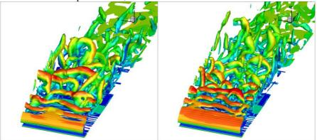
**Fig. 1:** Comparison of instantaneous iso-surface of Q-criterion: Baseline (left) and fine mesh (right).
