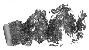
Fig. 1. Visualization of the flow over circular cylinder simulated by IB approach.
