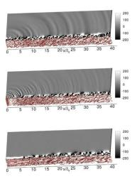
Fig. 1 Iso-Q criterion (Q=0.25  $U_0^{2}/\delta_0^{2}$ ) coloured by sign( $\omega_x$ ), instantaneous pseudo-dilatation field (gray scale). SEM (top), white noise (middle), new ZIBC-based approach (bottom).
