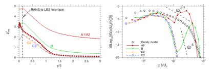
Fig. 2 Resolved pressure fluctuations in a flat-plate zero-pressure-gradient turbulent boundary layer at  $Re_{\theta} = 5200$ . Left: rms profile; right: power spectral density of wall pressure. Cases A: SEM, B: white noise, C: present new ZIBC-based approach.
