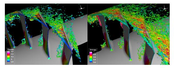
Figure 1. Tip clearance flow in a compressor rotor (Left: DDES model; Right: SLA-DDES model)
