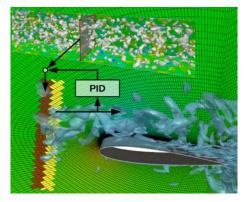
**Fig. 2** Synthetic turbulence is introduced by a volume force field and adjusted within a control loop.
