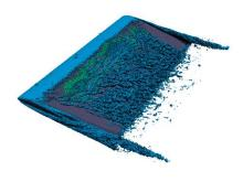
**Fig. 1** Wing with separation region (green iso-surface) and iso-surfaces from Q-criterion (blue).
