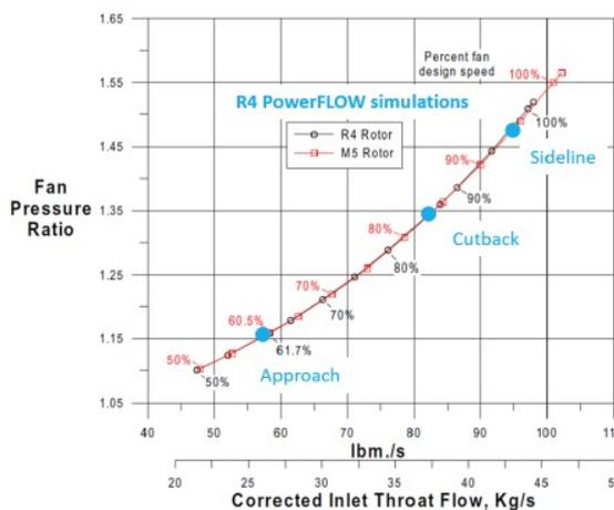
**Figure 4: Measured and predicted fan stage performances for the baseline configuration (R4 rotor).**
