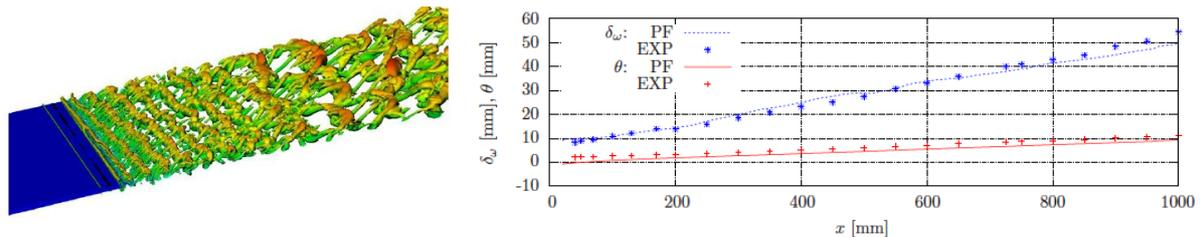
Figure 1: PowerFLOW simulation of shear layer mixing problem from Ref. [7]. On the left iso- $\lambda_2$  surfaces and on the right vorticity and momentum thickness downstream the trailing edge.
