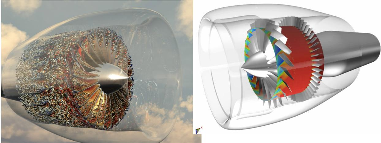
**Figure 3: PowerFLOW prediction of turbulent flow structures in the NASA SDT engine at approach conditions (left) and shock structures at take-off conditions (right).**
