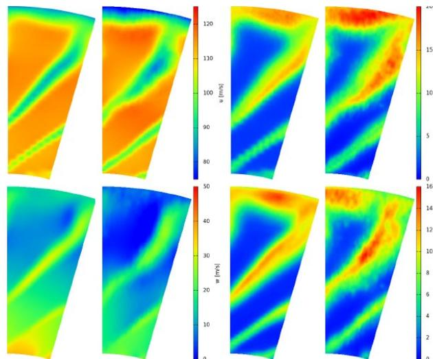
**Figure 5: Phase-locked average (left block) and SDV velocity (right block) at station #1 for the baseline OGV [m/s]. Axial (top) and radial velocity (bottom). Measurements on the left, simulations on the right.**
