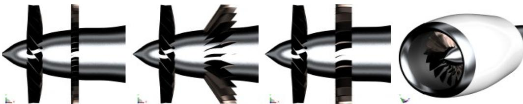
Figure 2: NASA SDT fan stage configurations. From left to right, baseline, low-noise and low-count OGV, and nacelle.
