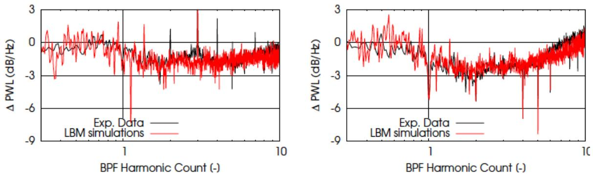
**Figure 6: Relative PWL at sideline conditions. Low-Count/Baseline (left) and Low-Noise/Baseline (right).**
