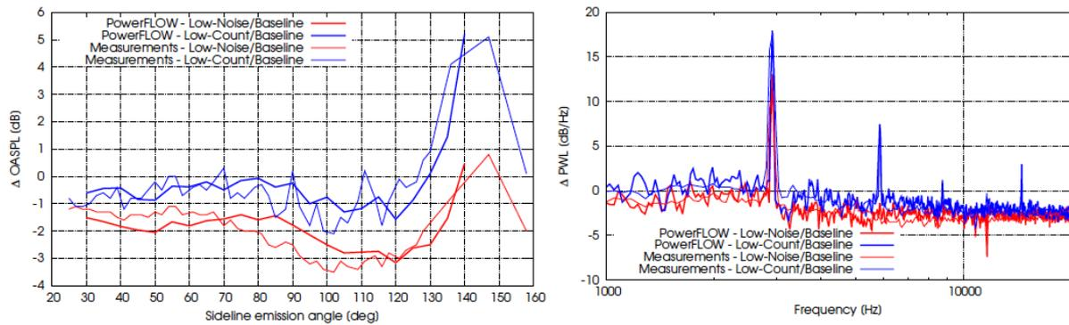
**Figure 6: Relative noise levels at approach conditions. OASPL (left) and PWL (right).**
