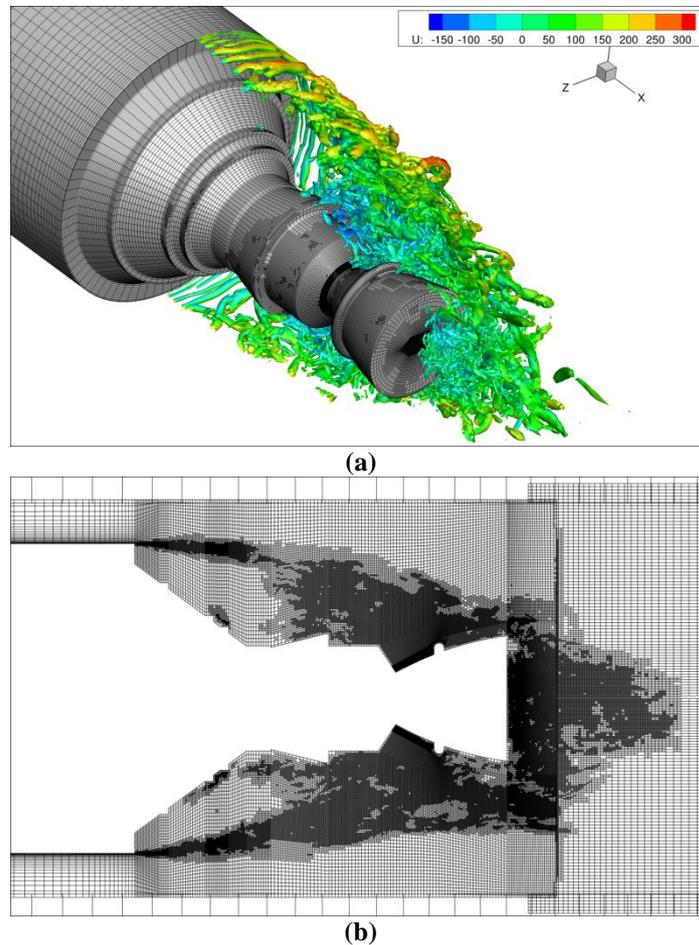
**Fig. 1** Ariane 5 model buffeting using a  $k - \varepsilon$  HRL model and an AMR method. (a): Q criterion colored by axial velocity. (b): slice of the AMR overset meshes in the recirculation area
