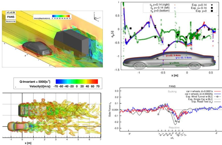
Figure 3: “On-road” overtaking maneuver: instantaneous streamline pattern and corresponding iso-contours of the mean velocity magnitude (upper left), pressure distribution over the car top and underbody surfaces (upper right), flow field visualized by the Q-criterion ( $Q = 5000 \text{ s}^{-2}$ ) (lower left) and variation of the car-related aerodynamic coefficient associated with the side force  $C_s$  (lower right)
