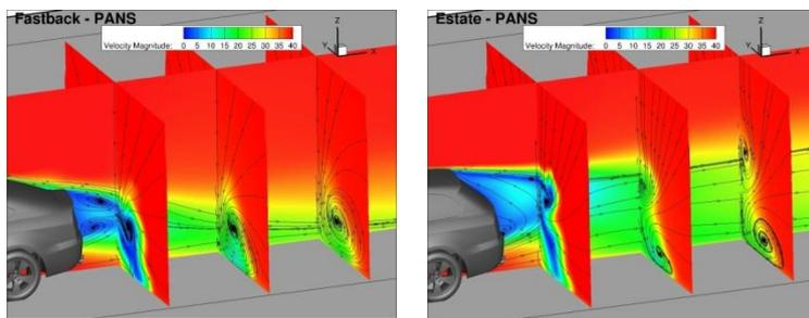
Figure 2: Time-averaged streamline patterns in the wake of the DrivAer car model in terms of different rear end shapes colored by the magnitude of the axial velocity component
