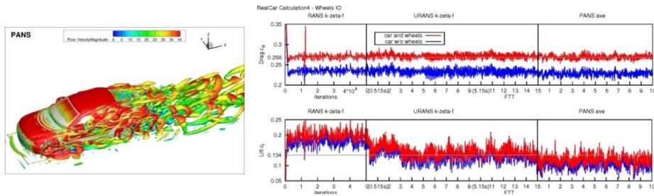
Figure 1: Flow past a BMW car model: (left) flow field visualized by the Q-criterion ( $Q = 5000 \text{ s}^{-2}$ ) and (right) history of the drag and lift coefficients obtained by RANS, URANS and PANS.
