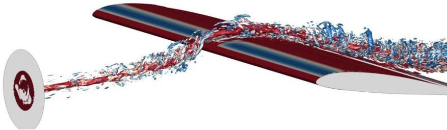
**Fig. 1:** Resolved vortex traveling downstream along the upper side of the HGR01 airfoil. The boundary layer is treated in RANS mode.
