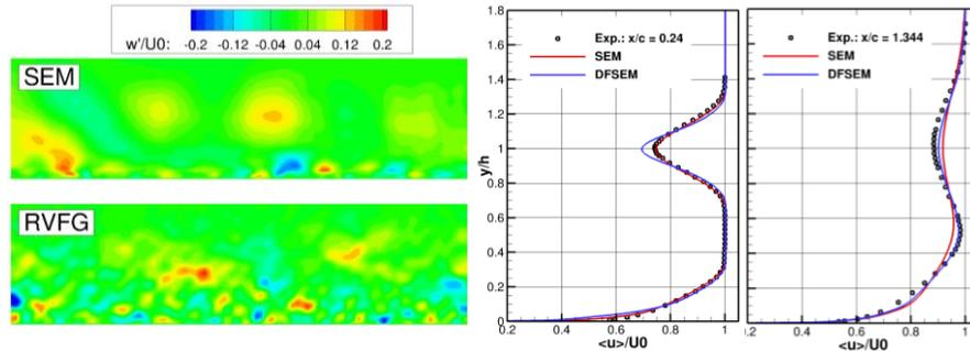
**Fig. 1** *Left:* Lateral synthetic fluctuations in the flat-plate boundary layer at  $Re_\theta = 3000$ . *Right:* Mean velocity profiles in the mixing co-flow.
