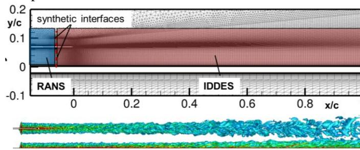
**Fig. 2** Mixing co-flow: Simulation setup and Q-criterion from DFSEM.
