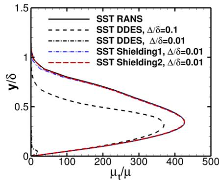
Figure 1: Eddy-viscosity ratio in a flat-plate boundary layer for different grid spacing to boundary-layer height ratios. Comparison of RANS, DDES and new shieldings
