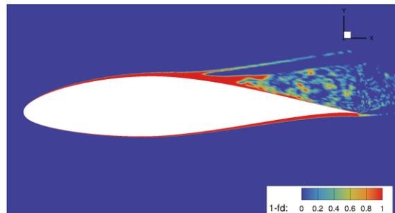
Figure 2: Application of the new shielding function to a stalled airfoil
