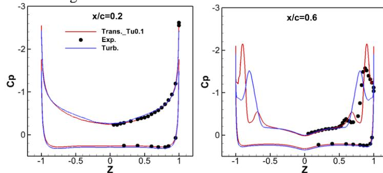
Fig. 1 Pressure coefficients on different sections along streamwise direction.
