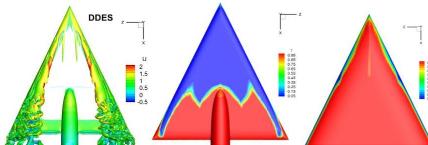
Fig. 2 Left: isosurface of  $Q$  criterion; The distribution of intermittency factor  $\gamma$  on the surface of VFE-2.(Middle: windward; Right: leeward.)
