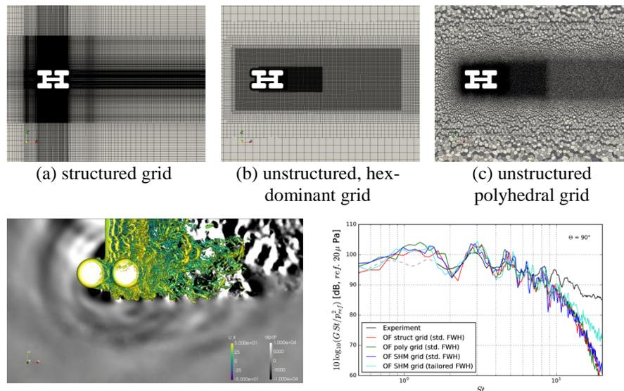
**Fig. 1** Application of grey-area improved  $\sigma$ -DDES model to aeroacoustics of a rudimentary landing gear on different grid types (top), unsteady flow field and acoustic farfield spectra at observer location  $\theta = 90^\circ$  (bottom).
