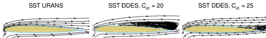
**Fig. 1** In-plane streamlines at 77 % rotor radius at  $t/T = 0.43$  (upstroke) indicate grid-induced trailing edge separation with DDES and influence of empirical constant  $C_{d1}$ .
