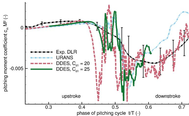
**Fig. 2** Influence of empirical constant  $C_{d1}$  of SST-DDES on local pitching moment during dynamic stall on a model rotor blade.
