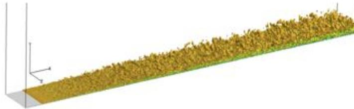
**Fig. 1.** Resolved turbulent structures visualised by an iso-surface of the second invariant of the velocity gradient, coloured by streamwise velocity, from [6].
