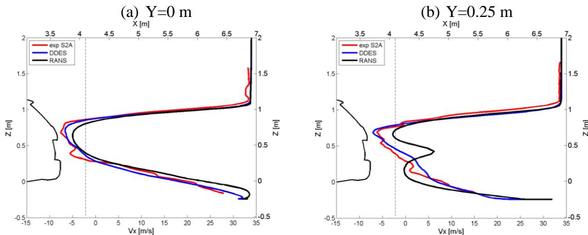
**Fig. 2:** Streamwise velocity profiles  $V_x$  in the wake of the simplified estate shape without wheels, 400 mm behind the body
