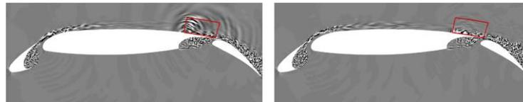
**Fig. 3** Instantaneous pseudo-dilatation field around a high-lift configuration using white noise forcing on the left and the new ZIBC-based approach on the right
