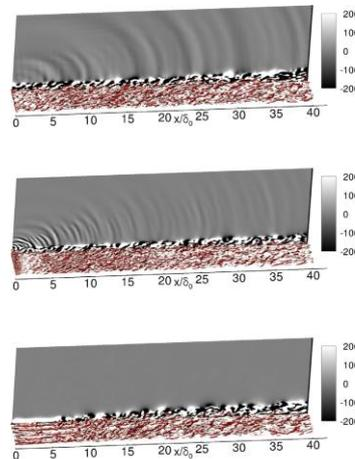
**Fig. 1** Iso-Q criterion ( $Q=0.25 U_0^2/\delta_0^2$ ) coloured by  $\text{sign}(\omega_x)$ , instantaneous pseudo-dilatation field (gray scale). SEM (top), white noise (middle), new ZIBC-based approach (bottom).
