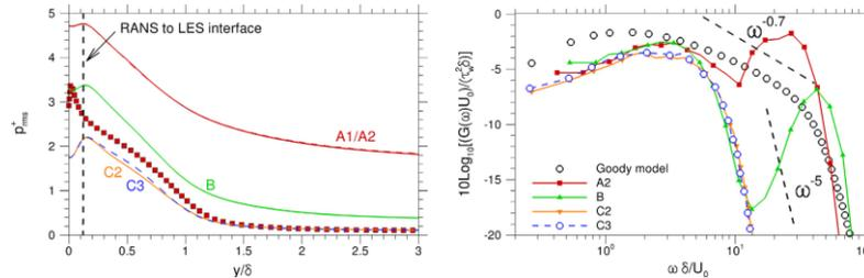
**Fig. 2** Resolved pressure fluctuations in a flat-plate zero-pressure-gradient turbulent boundary layer at  $Re_0 = 5200$ . Left: rms profile; right: power spectral density of wall pressure. Cases A: SEM, B: white noise, C: present new ZIBC-based approach.
