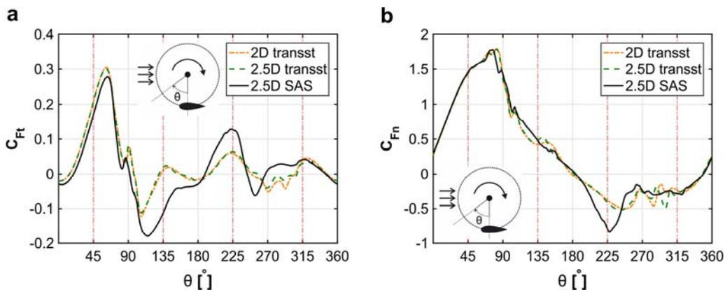
Figure 1. Tangential and normal force coefficients during the last turbine revolution.
