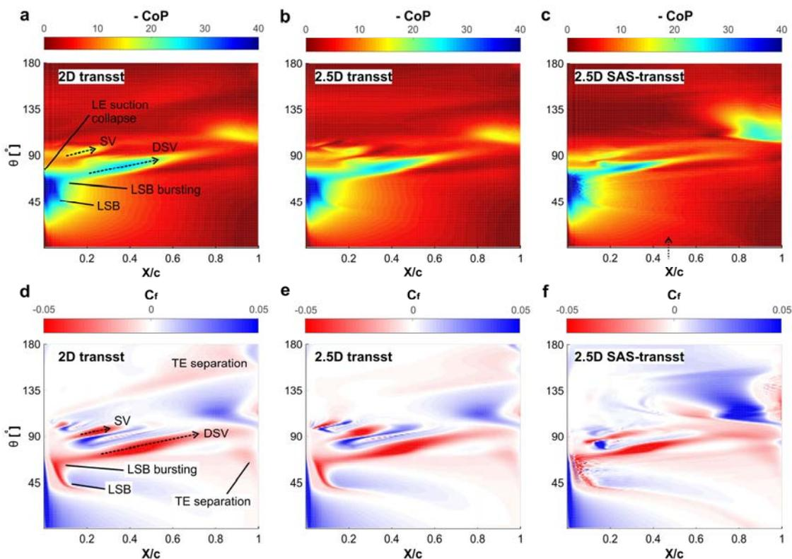
Figure 2. Spatiotemporal distribution of coefficient of (a-c) pressure and (d-f) skin friction over the blade suction side in the fore half of the last turbine revolution. 'LE', 'TE', 'LSB', 'DSV', 'SV' denote 'leading edge', 'trailing edge', 'laminar separation bubble', 'dynamic stall vortex' and 'secondary vortex', respectively.
