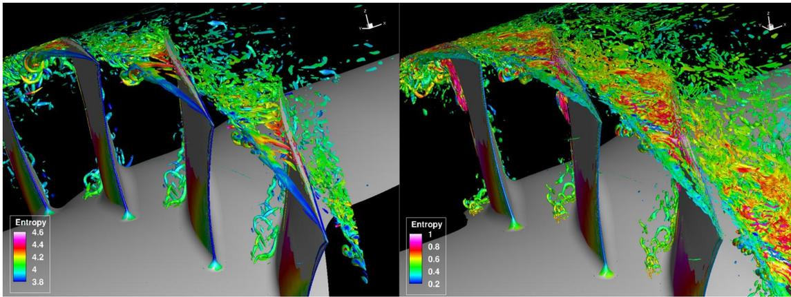
Figure 1. Tip clearance flow in a compressor rotor (Left: DDES model; Right: SLA-DDES model)
