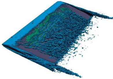
**Fig. 1** Wing with separation region (green iso-surface) and iso-surfaces from Q-criterion (blue).
