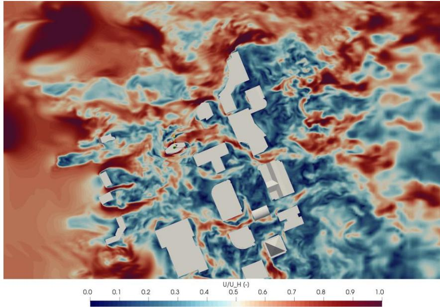
...**Fig. 1** Contours of relative velocity on a plane 40m above the ground (full scale)
